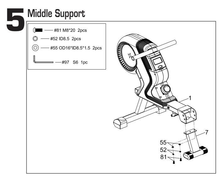
Attach the Middle Support (7) to the Main Frame (1). Secure using 2 Screws (81), 2 Spring Washers (52) and 2 Washers (55) with the provided Allen Wrench (97).
