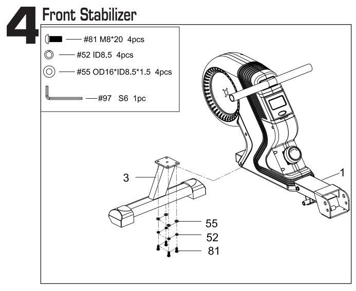
Attach the Front Stabilizer (3) to the Main Frame (1). Secure using 4 Screws (81), 4 Spring Washers (52) and 4 Washers (55) with the provided Allen Wrench (97).
