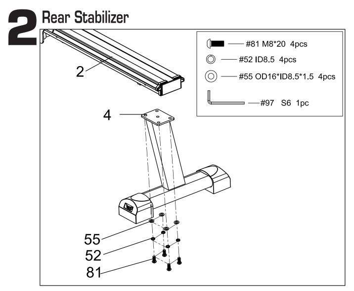
1. Attach the **Rear Stabilizer (4)** to the **Slide Rail (2)**. Secure using 4 **Screws (81)**, 4 **Spring Washers (52)** and 4 **Washers (55)** with the provided **Allen Wrench (97)**.
